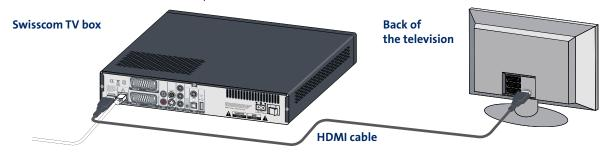
Connect the Swisscom TV box to the power outlet and switch it on using the switch on the back. The Swisscom TV box loads and installs the latest version of the Swisscom TV software during commissioning. This process takes 30 minutes. It is completed when the clock on the display shows the correct time. Please do not switch off the Swisscom TV box!
