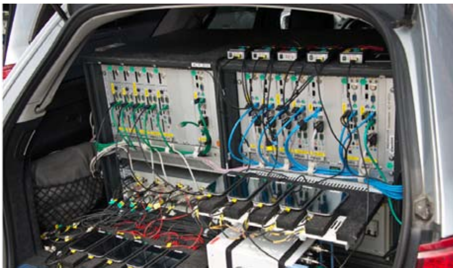
Measurement equipment of one of the two cars establishing the mobile to mobile calls.
