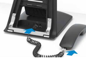
The cable end with the longer straight cable piece is connected to the phone , the other end to the handset.
