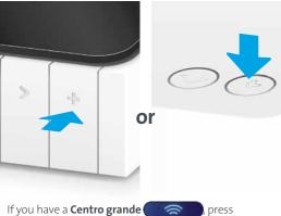
Without delay, press for 2 seconds on the WPS button on your repeater. The WLAN LEDs start blinking green.
