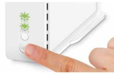
Wait ca. 2 minutes until the WLAN LEDs stop blinking. If the LEDs start blinking red, repeat steps 3 and 4.
