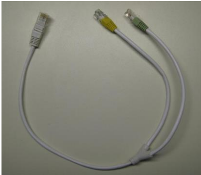
Figure 14: Example of Y cable, signals for the DSL socket DD (pin 4 and 5; pin 3 and 6) for NTE: DSL and FXS
