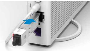
Push in the fibre optic module into the «fibre» insert until it clicks in. The red markings on the fibre optics module (bracket) and Internet-Box belong on the same side.
