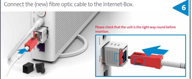
Remove the protection caps and connect the red end of the cable into the Internet-Box. The cable is sensitive, so please do not touch it at either end!
