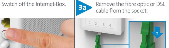
Remember the slot number. Press the lever against the plug (1). The cable can then be pulled out easily (2).
