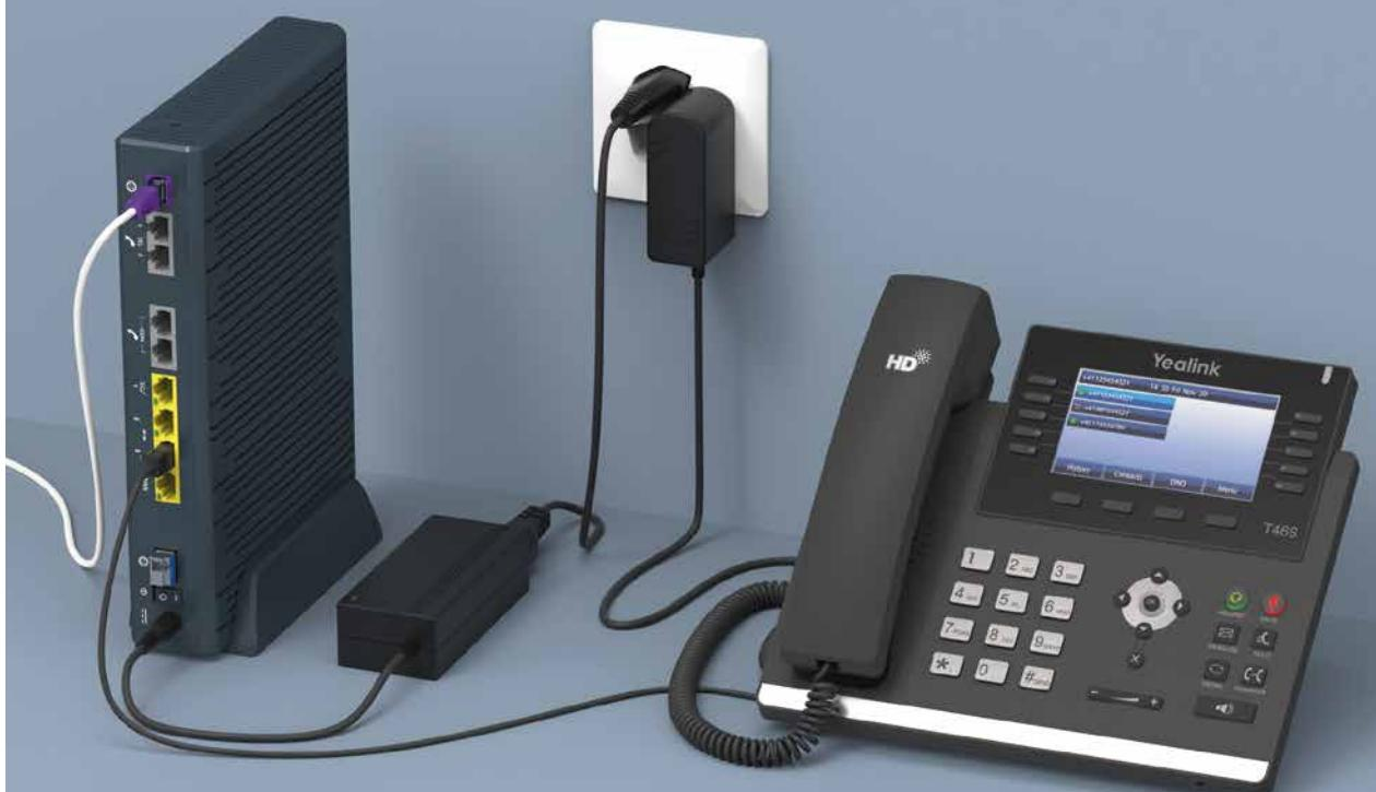
**4** Connect the phone to the router using the supplied Ethernet cable.
