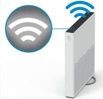
You can activate and deactivate your WLAN by pressing the 🕿 button. You will find further information about your WLAN as well as your access data (WLAN name and password) on the reverse side of this manual. (4)
