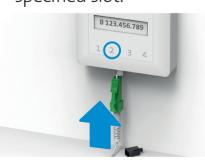
Only one slot works: Remove the protective cap. Open the slot specified by the letter on the fibre-optic socket (usually «2», sometimes «1»).
