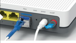
Do not dismantle old installation until the new Internet-Box is set up successfully. Reset the Internet-Box to its factory
