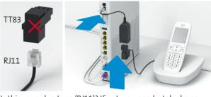
Is this your plug type (RJ11)? If not, you need a telephone adapter RJ11/TT83 (swisscom.ch/connectionaccessories).
