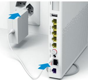
**5** Connect the DSL cable to the white adapter.
