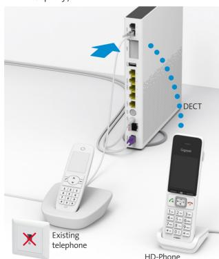
Select the connection mode in the settings of your HD-Phone and press the +button on your Internet-Box. The two devices connect automatically.
