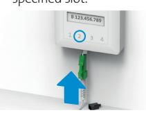
Only one slot works: Remove the protective cap. Open the slot specified by the letter on the fibre-optic socket (usually «2», sometimes «1»). Note: If your slots are facing upwards, slot 2 is the second
