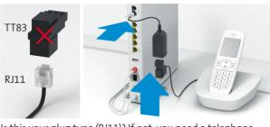
Is this your plug type (RJ11)? If not, you need a telephone adapter RJ11/TT83
