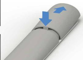
To open the remote control battery compartment, press down on the back of the cover with your thumb and slide it away from you.
