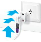
c) Only once you have installed this telephone socket (digital socket) can you use all telephone sockets in your home for your phones and fax machines. Without this telephone socket you have to plug your phones/fax machines directly into the Internet-Box, connect or have your home installation adjusted by a service
