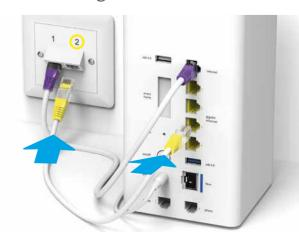
«2») and the Ethernet-Switch with an Ethernet cable.
