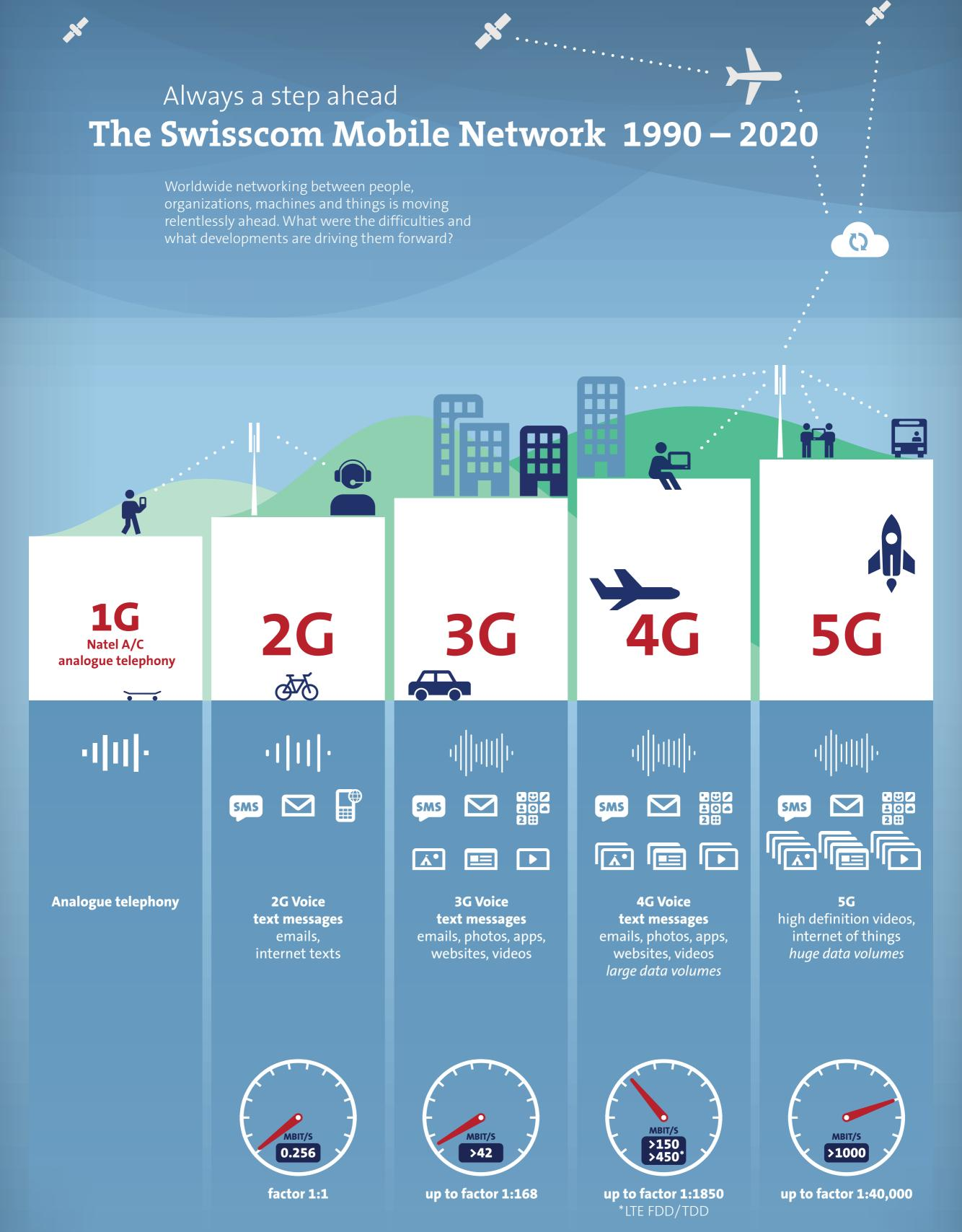
**5G** will provide  $\overline{a}$  40,000 times more  $\overline{rap}$  id data transmission rate
