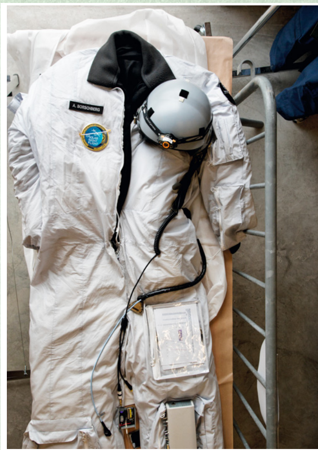
The aircraft has no heating or air-conditioning system, so the pilot needs a THERMAL SUIT . This offsets the extremes of temperature in the cockpit, between +40 and -20 degrees, by inflating or deflating as the pilot presses a button.
