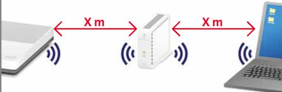
**N.B.** Place the repeater at an equal distance between the router and the place that lacks WiFi coverage.
