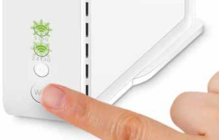
Wait ca. 2 minutes until the WLAN LEDs stop blinking. If the LEDs start blinking red, repeat steps 3 and 4.
