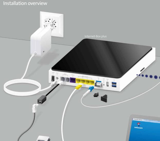
Connect the new fibre optic cable to the Internet-Box.
