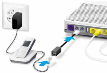
**Internet-Box** (phone 1 and 2) – and not the telephone socket as before. Use the black telephone adapter if necessary.
