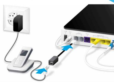
**Now only** connect your telephone and/or fax machine **to the Internet-Box** (phone 1 and 2) — and not the telephone socket as before.
