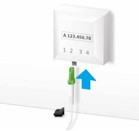
Open the slot on the fibre optic socket that we specified to you per letter. This is generally slot 2, rarely slot 1. Remove the protective cap and connect the **green** cable end.
