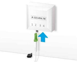
Open the slot on the fibre optic socket that we specified to you per letter. This is generally slot 2, rarely slot 1. Remove the protective cap and connect the green cable end.
