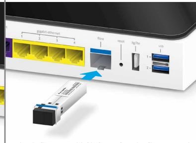
Push in the fibre optic module (clip facing up) into the «fibre» insert until it clicks in.
