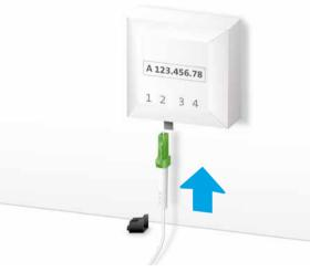
On the fibre optic socket open the slot we specified in our letter. This is usually slot 2, seldom slot 1. Remove the protective cap and connect the green end of the cable.
