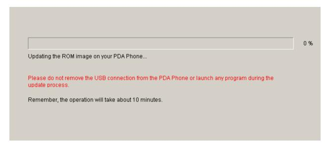
The progress bar may stop moving during the upgrade. This is normal as the RUU is adjusting itself in order to complete the update process automatically.
