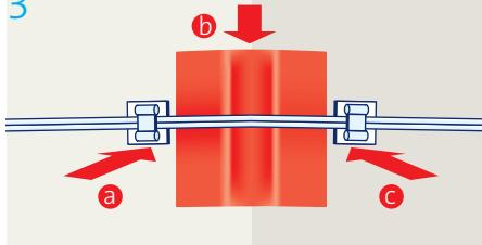
When laying the cable around corners, use the corner template. Refer to steps **a** to **c**. Remove template.
