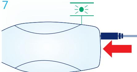
Connect both media converters to the power supply using the mains adapter.
