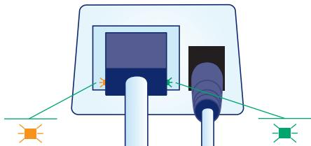
Check connections: LEDs on the Ethernet connectors must flash orange and green. In the event of any disruption, see reverse side.
