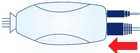
Connect both media converters with Ethernet cables to DSL modem and Swisscom TV-Box or computer.
