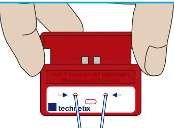
Cut both ends of cable for optimum connection. Use the upper opening on the cutter to do this.
