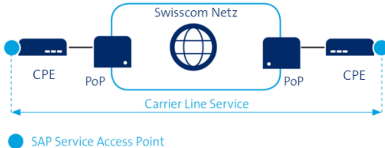
Figure 2: Graphical representation of a Carrier Line Service Basic / Premium Silver
