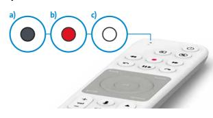
a) The LED does not light up when you use the remote control.
