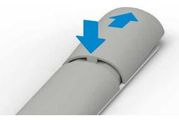
To open the remote control battery compartment, press down on the back of the cover with your thumb and slide it
