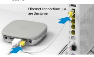
**Do not yet** plug in the power supply for the Swisscom Box. For information on how to connect wirelessly, please refer to the back page of this leaflet. (1)
